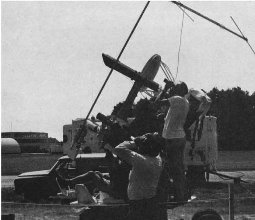
Tom Rankin assists in tracking Walt Good's Soaring Glider by standing on electrically driven binocular mount. Pilot sits behind the long binoculars and Optical Tracker sits below him, aiming the Tracker like a machine gun. Maynard's Yagi beam antenna is seen at the top of the photo. It works well.
